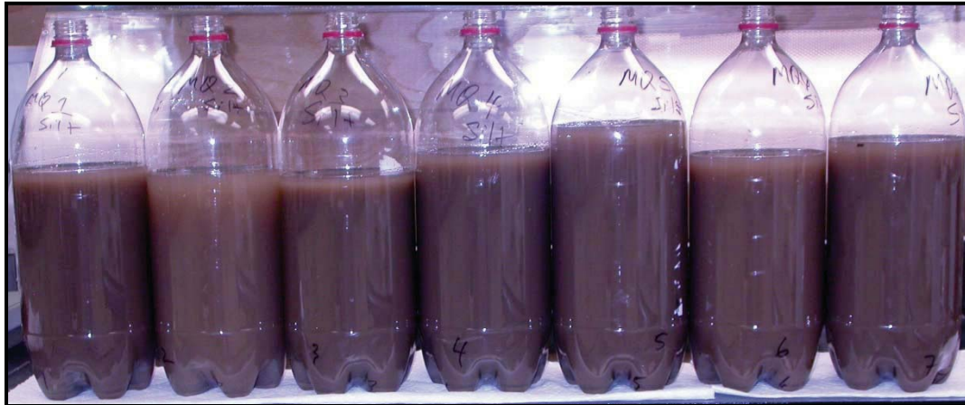
Figure E-7. During Clay Removal. The clay remains suspended while the larger silt particles settle out.
