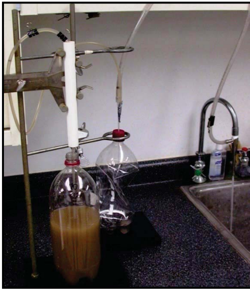
Figure E-9. Aspiration was Used to Generate Vacuum to Siphon the Clay Solution from the Sample Container. The white tube keeps the transfer line vertical (the solution pick-up line is Tygon® tubing with a 2 ml. glass pipette on the end). The binder clip on the tubing above the white tube keeps the pipette suspended the correct distance above the silt bed. The withdrawn clay fraction solution is collected in the receiving bottle (right) via vacuum, allowed to settle, and the entire clay fraction later recovered and dried.
