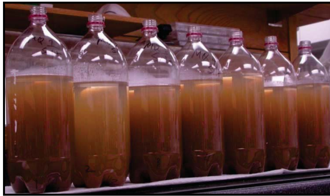
Figure E-10. The Silt/Clay Mixtures Nearing the End of Removal of the Suspended Clay Fraction (the silt and remaining clay is repeatedly re-suspended and allowed to settle to enable removal of as much clay as possible).
