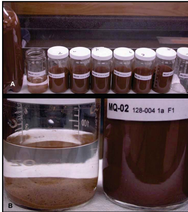
Figure E-5. Removal of Silt and Clay from the Sand Fraction The suspended small (i.e., < 50 micron) particle fractions were transferred to a 2-liter container for future processing (A, see far left [edge of funnel and bottle are visible]). Following complete silt/clay fraction removal, only the sand remained behind (B, left, 2Akb sample). The Feature 1 soil sample (B, right) still has all three soil fractions present (i.e., sand, silt, and clay) prior to decanting.
