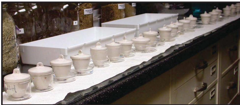
Figure B-3. Crucibles containing silt fractions ready for ashing in the muffle furnace to remove organic materials.
