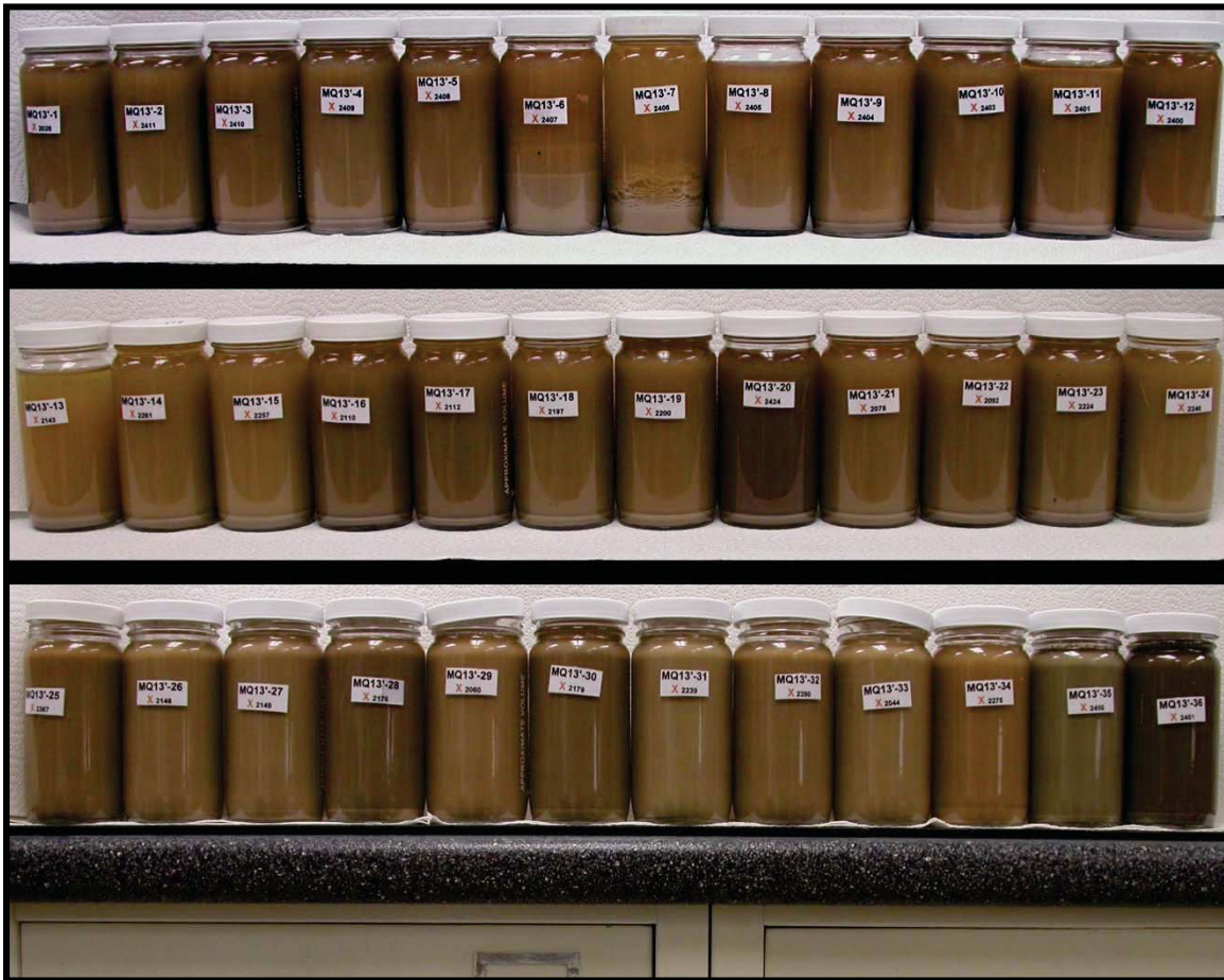
Figure E-2. Silt clay fraction solutions prior to first aspiration from 250 ml sample bottles. Note incomplete settling visible in the middle two bottles in the top row. Also note the drastic difference in appearance of the two surface control samples (bottom row, last two bottles). The above samples are in the same order as listed in Table E-1.
